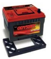
Optional height adapter may be used on the 34-PC1500 for installations where a group 24 or group 27 is required. Snap the adapter securely into place on the bottom of the 34-PC1500 battery. In some installations, a 34-PC1500 with this adapter may be used to replace a group 24F or 27F depending on required cable length.
